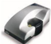
Zetasizer Nano ZSP Protein size and charge, electrophoretic mobility, molecular weight, B_{22} , k_D
